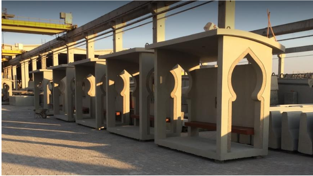
Figure 3.1: Image taken showing majority of precast works being modular units at precast supplier production yard
