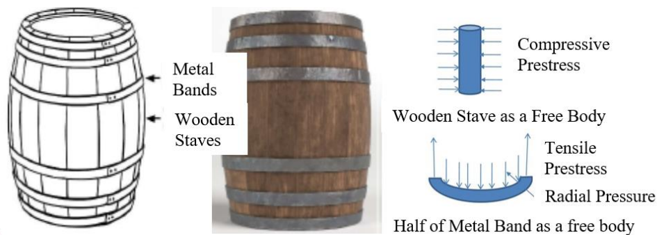
Figure 1.1 Prestressed barrel in the early ages and the general principle of prestressing applied to barrel construction (Neupane ,2020)
