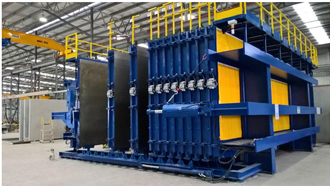
Figure 1.4: Molds used for Precast Concrete walls (Catalogue molds, accessed 28th July, 2021)
