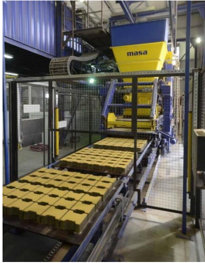
Figure 3.3 Interlock drainage tiles production chamber
